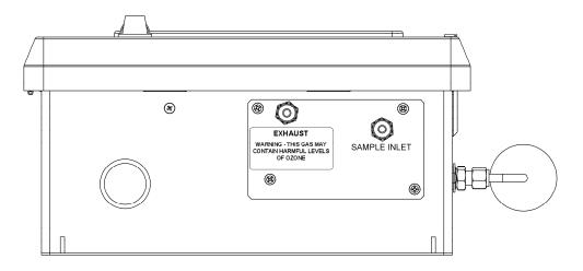
Figure 4-3: Pneumatic Connections, NEMA Configuration, Single Stream
